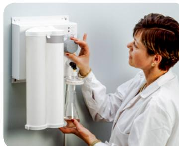
Dispense deionized water easily by simply turning the dispensing valve.
